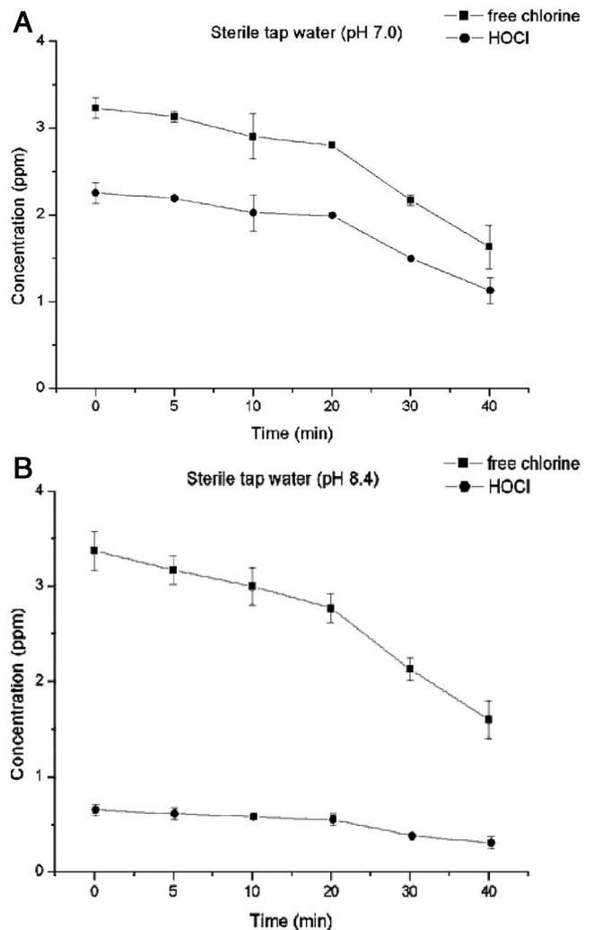
Fig. 1. Generation of free chlorine and HOCl in solution with pH 7.0 tap water (A) and pH 8.4 tap water (B).
